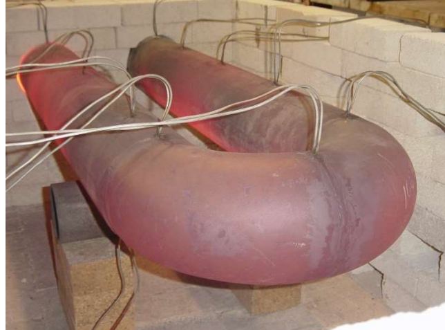
Figure 2 - Bio-Oil testing firing into a radiant tube in Bloom's lab
