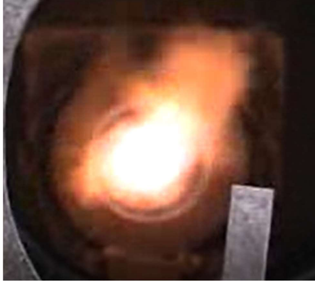
Figure 1 - 100% Methanol flame firing at roughly 15% excess air conditions
